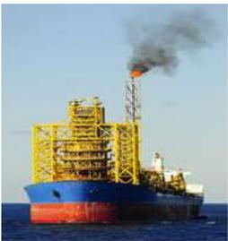
**Plataforma FPSO (Floating, Production, Storage, and Offloading):** Navios capazes de processar, armazenar e transferir petróleo e gás natural.
